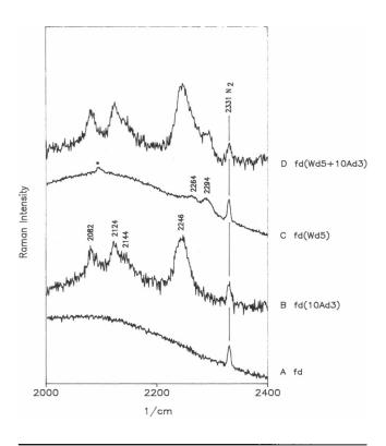
FIGURE 6 Raman spectra in the region 2,000–2,400 cm<sup>-1</sup> of: (A) normal fd, (B) fd( $10A_{d3}$ ), (C) fd( $W_{d5}$ ), and (D) fd( $W_{d5}$ +  $10A_{d3}$ ); obtained as indicated in Fig. 4. Spectral frequencies and intensities are scaled to the band at 2,331 cm<sup>-1</sup> in each spectrum which is due to ambient  $N_2$ . The asterisk (\*) indicates a laser artifact. All other bands are due to C-D stretching modes of deuterated side chains, as assigned in Table 1.
